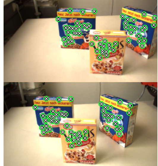
(b) Reprojection of the best map onto the images of left and right camera.
