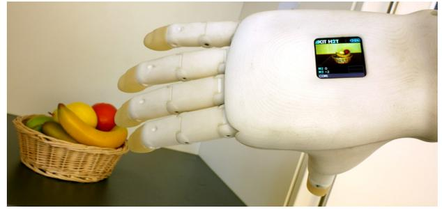
Fig. 5: Display mounted in the backside of the hand
