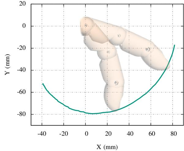
Fig. 8: Index finger trajectory
