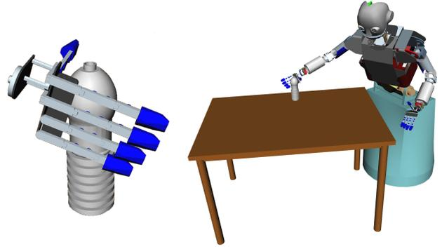
Fig. 5. The target object with grasp (left). An exemplary IK result with 13 DoF (right).
