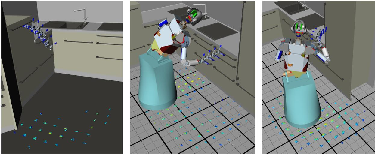
Fig. 6. A trajectory for opening the dishwasher with depicted *ORM* (left). The trajectory for opening the drawer with exemplary IK solution for the final pose (center). A trajectory for opening the fridge with robot configured at the final trajectory point (right).
