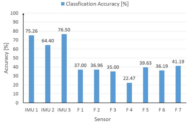
Fig. 4: Classification accuracies using single IMU or single force  $F$  sensors.
