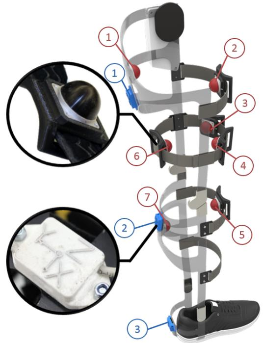
Fig. 1: Passive exoskeleton with 7 3D-force (red) and 3 IMU sensors (blue). The numbers correspond to the sensor labels.
