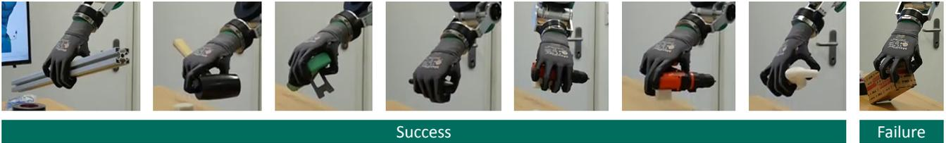
Fig. 9: Exemplary grasping results using the underactuated five-finger hand of ARMAR-6.
