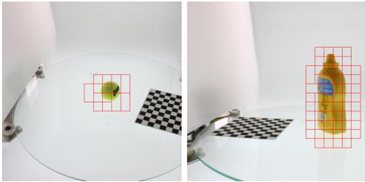
Fig. 4: The large input image is sliced into smaller images and reclassified. High confidence classifications are bounded.
