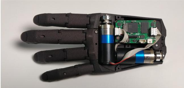
Fig. 1: KIT Prosthetic Hand (50<sup>th</sup> percentile female) with Zynq Z7010-based processing system
