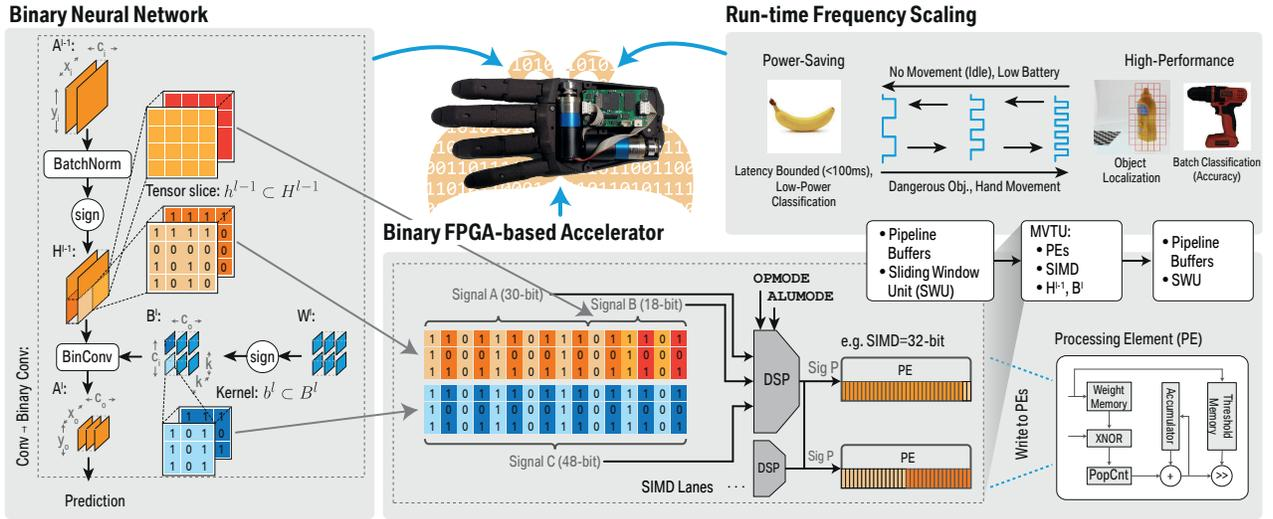
Fig. 2: Overview of Binary-LoRAX: BNN tensor slices are fed into DSPs which perform high-throughput XNOR operations. DSP results are forwarded to the PEs of an MVTU. A single MVTU of the pipeline is shown for compactness. Runtime frequency scaling allows high-performance functions, or power-saving mode.
