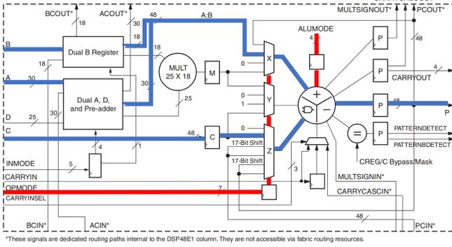
Fig. 3: The DSP48E1 Slice [41]. Appended blue path indicates the operands inside the DSP, red path indicates signals that are needed to achieve the desired binary mode.
