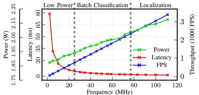
Fig. 5: Runtime frequency scaling ranging from 2MHz to 111MHz for the  $v$ -CNV prototype
