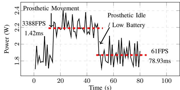
Fig. 6: Run-time change in operation mode based on application scenario, e.g. motion, delicate object or low battery
