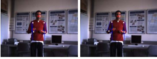
Fig. 6. Illustration of the effect of incorporating inverse kinematics. Left: without inverse kinematics. Right: with inverse kinematics.
