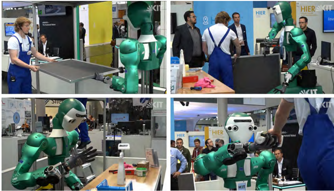
Fig. 10: During the CEBIT demonstrations, ARMAR-6 recognized the need of help as the technician carries out a maintenance task. ARMAR-6 and the technician lower and transport a guard cooperatively (top left) and place it at a place chosen by the human (top right). While the technician inspects the conveyor belt, ARMAR-6 brings necessary cleaning equipment from the workbench (bottom left). The handover based on human pose tracking allows the technician to comfortably receive the equipment (bottom right).
