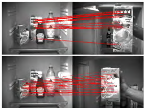
Fig. 9. Scene analysis in a refrigerator: the traces visualize the correspondences of the local features between the learned view and the current view.
