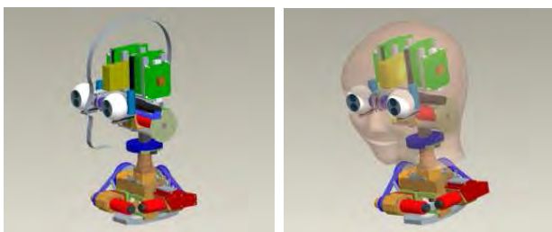
Fig. 3. Rendering of the head/neck system: Two cameras per eye. The eyes have a common tilt and can pan independently. The visual system is mounted on a 4 DOF neck which is realized as a Pitch-Roll-Yaw-Pitch mechanism.
