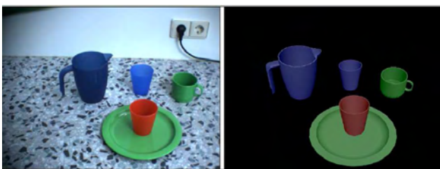
Fig. 8. Typical result of a scene analysis. Left: input image of the left camera. Right: 3D visualization of the recognition and localization result.
