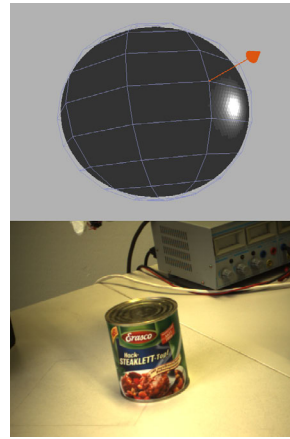
(b) Resulting saliency sphere and foveal view for the soup can search task.
