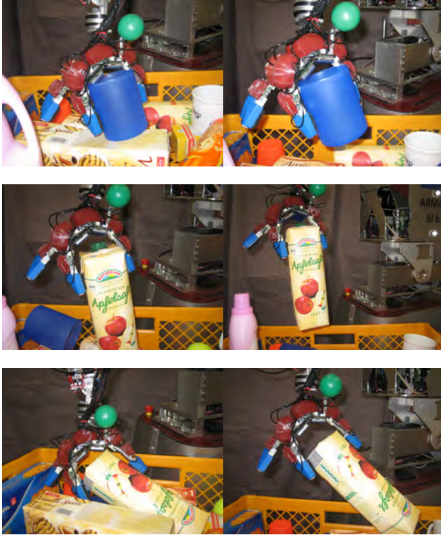
Fig. 6: Some example grasps. Left column: situation immediately after closing the hand. Right column: After lifting the object.
