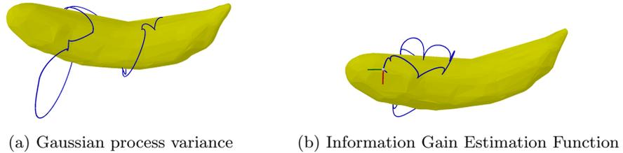
Fig. 6: Exemplary exploration progress of the YCB banana. The blue line depicts the complete trajectory during the exploration. Following the GP-V leads to long jumps across the surface resulting in a high travel cost (left). The targets generated by the IGEF approach lie closer together forming a dense pattern with short hops between contact points (right).
