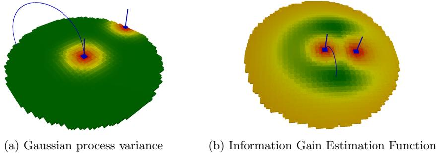
Fig. 4: Predicted information gain after the second contact on a flat surface. The Gaussian process variance approach suggests a target that lies on the edge of the allowed area (left). The IGEF based strategy prefers a target that is closer to the existing contacts to minimize path cost (right). The trajectory to the next best touch target is depicted as a blue curve.
