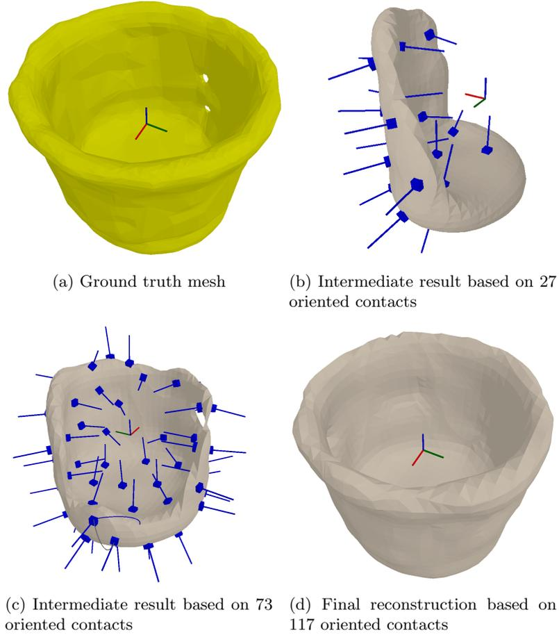
Fig. 8: The IGEF-based approach leads to a complete and cost-aware exploration of an unknown object (YCB object nr. 25)
