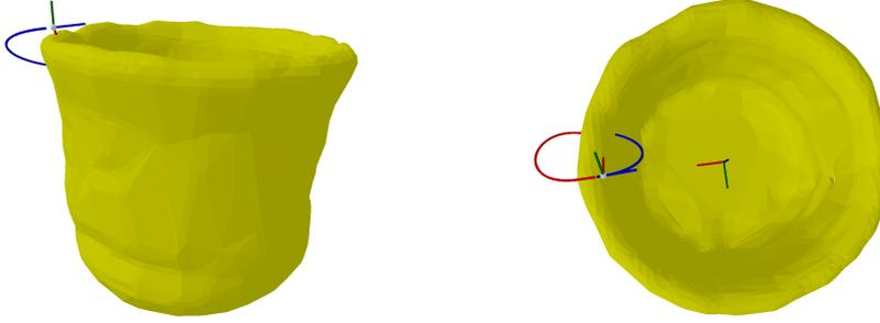
Fig. 3: Example trajectory of a missed edge. The predicted surface contact does not lie on the actual object surface and thus the calculated trajectory misses the object (left). The trajectory is continued to re-establish contact with the object by approaching the previous contact (right).
