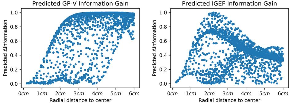
Fig. 5: Predicted information gain after several contacts. The GP-V approach rates multiple targets close to the maximum rating of 1 (left) while IGEF suggests a maximum rating of 1 only in a small region (right).
