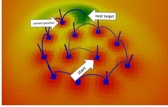
Fig. 2: Exemplary exploration of a flat plane. The combination of the exploration goals  $\Psi_1, \Psi_2$  and  $\Psi_3$  leads to an exploratory path that roughly follows an outward spiral. In green areas the predicted information gain is high, in red areas it is low.
