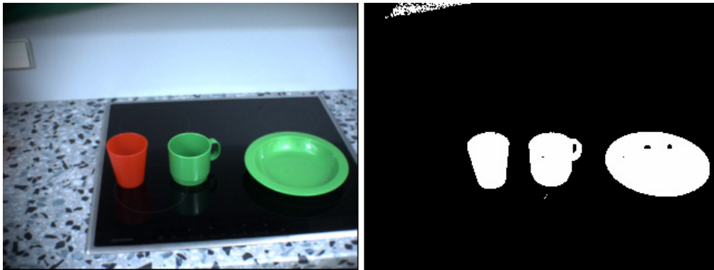
Figure 10: Illustration of the color segmentation result for the colors red and green
