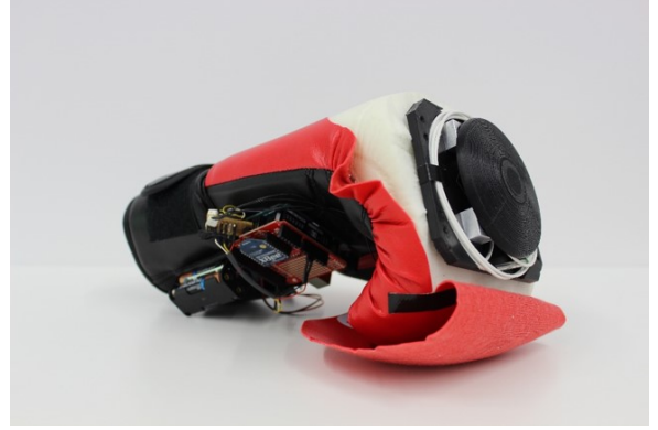
Figure 1 The force sensing glove, equipped with a piezo-resistive load cell, a microcontroller and a wireless down-link for data transmission. The leather cover is folded back to expose the sensor.
