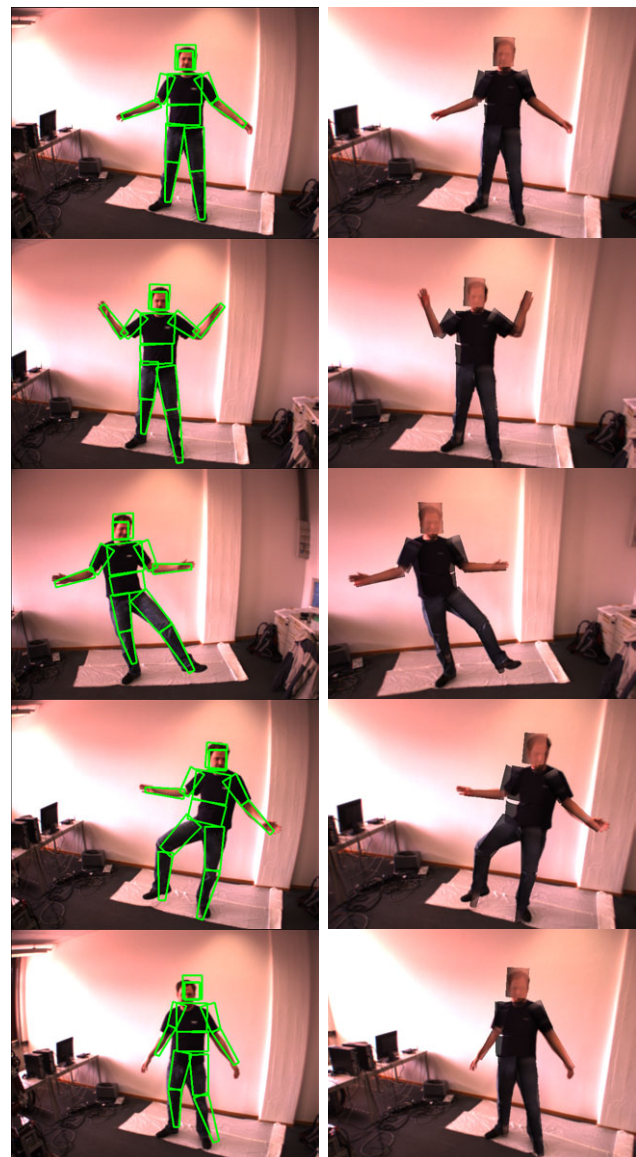
Fig. 6. A series of pictures from a tracking session. The left side shows the simplified cylinder projection, while the right side shows a 3D overlay over the rectified image. The 3D model is transparent and uses the color from the appearance model. The head and torso color are derived from the left arm.
