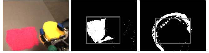
Fig. 3: Left: Robot view on the scene. Center: Segmented view of the scene in the beginning of the wiping execution. Right: Segmented view on a "clean" table.
