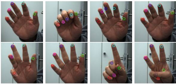
Figure 3. Images of the tracking results. Upper row: Simultaneous closing of the fingers. Lower row: Sequential flexing of the fingers. Labeling of fingertips: Thumb (green), index (light blue), middle (dark blue), ring (pink), and pinkie (red).
