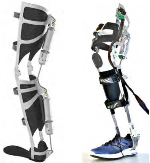
Fig. 1. The KIT exoskeleton consists of two active DOFs in the knee and the ankle. CAD design (left) and first prototype (right)
