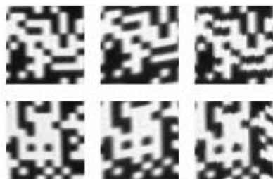
Fig. 4. Two local sample patterns for demonstration of the Gruen Algorithm; each left pattern in a row is a template pattern, each middle one is the actually captured pattern (distorted by scene geometry) and each right one is the pattern after application of the Gruen Algorithm
