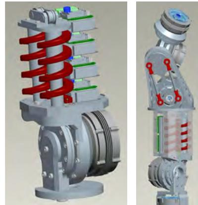
Fig. 8. The knee joint: The same driving unit is used with parallel springs.
