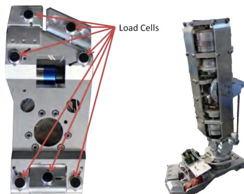
Fig. 10. Distribution of the load cells in the foot (left) and assembly of the lower leg and the ankle joint (right)
