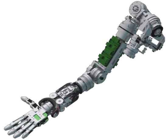
Fig. 4. 8 DOF arm of ARMAR-IV: In addition to classical 7 DOF humanoid robot arms, an additional DOF of the inner shoulder joint was realized according to the human arm model developed in [24] and based on manipulability analysis [25] to improve dexterity in particular in the case of bimanual manipulation.
