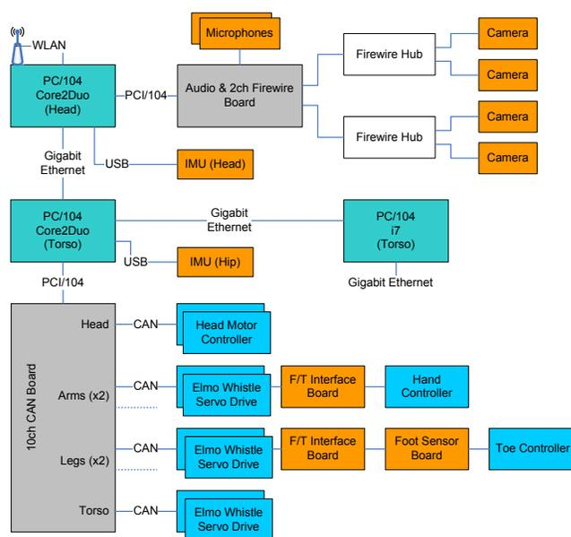
Fig. 11. Computer architecture of ARMAR-4
