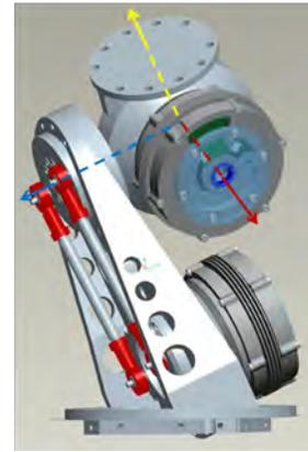
Fig. 7. The hip joints: All three joints intersect in a single point and are coupled to achieve the required high torques.
