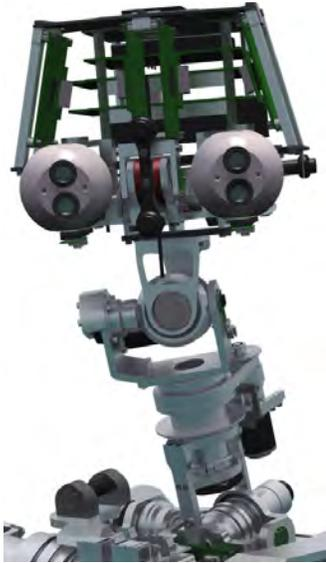
Fig. 3. 9 DOF head of ARMAR-IV: independent eye pan and tilt, lower and upper pitch, lower and roll and yaw. For cameras and six microphones.
