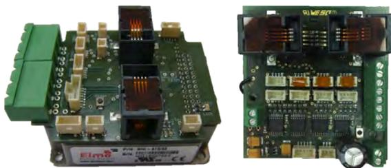
Fig. 9. Elmo Whistle Servo Drive with custom PCB (left) for control of one BLDC motor and the DC motor controller (right), which can control up to 4 DC motors.
