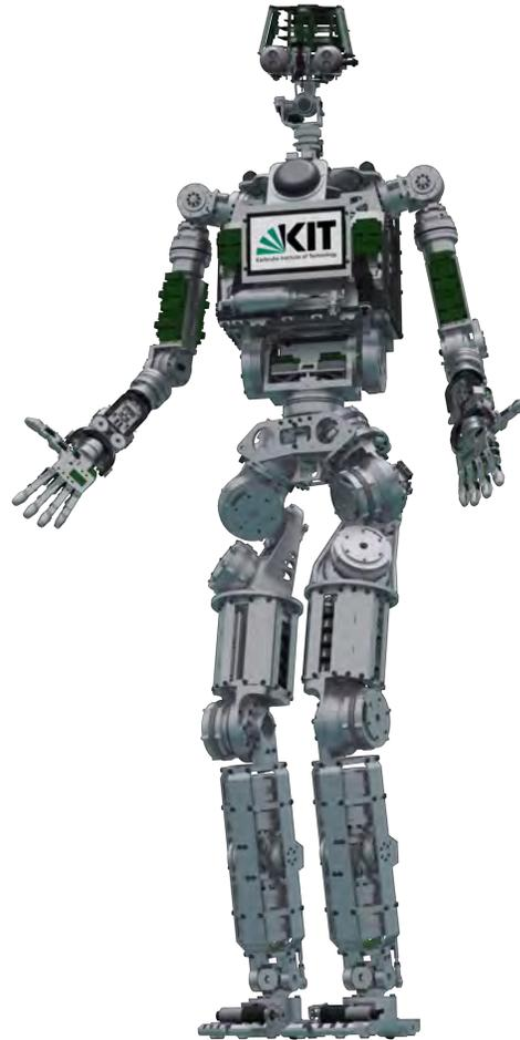
Fig. 1. The humanoid robot ARMAR-4: torque controlled humanoid robot with 63 active degrees of freedom, 63 actuators, 214 sensors, 76 microcontroller, 3 PCs, 70 kg and 170 cm.
