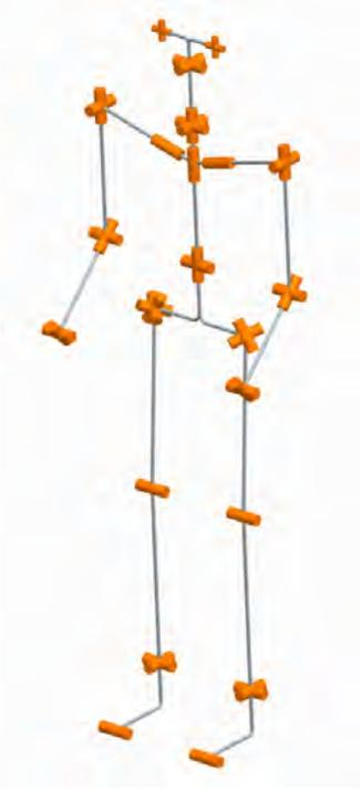
Fig. 2. The kinematic structure of ARMAR-4: head with 9 DOF, each arm with 8 DOF, each leg 7 DOF, hip with 2 DOF and each hand with 11 DOF (not shown in the figure)
