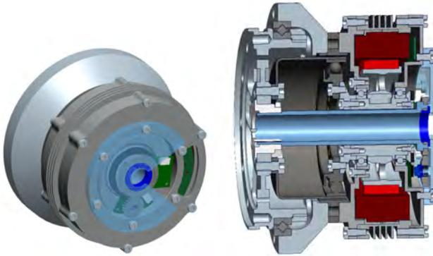
Fig. 6. Driving unit integrating motor, gear, incremental and absolute position sensors, torque and temperature sensors. To reduce costs, the design of the unit was optimized to reduce the number of mechanical parts resulting in only 11 mechanical parts needed to produce the driving unit.
