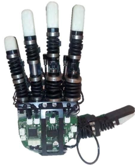
Fig. 5. 11 DOF humanoid hand actuated by fluidic actuators. The actuators are connected to on-board over pressure and under pressure tanks to allow fast and controlled closing and opening of the fingers
