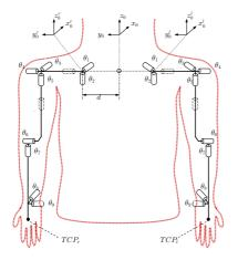
Fig. 4. The kinematics model of both arms
