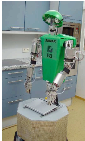
Fig. 1. The humanoid robot ARMAR with five subsystems: head, two arms, torso and mobile platform.
